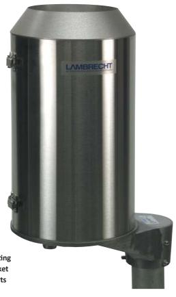
A uniquely brilliant idea... lies behind the sensor (1518 H3). Not only are collecting and drain funnel heated, but also the collecting ring. Here, the snow is thawed so that the snow fall is measured promptly. The new electronically regulated threecircle heating device minimizes evaporation effects. Several thousand of these sensors are in use world-wide.
