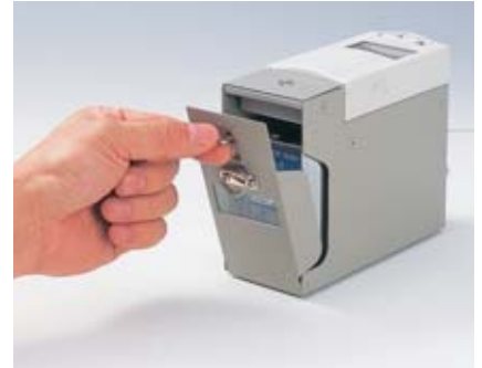
Lift the snap lock and open the sensor cover.
