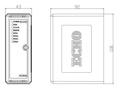
Fig. C- 3 HC104 Module Panel and Dimension
