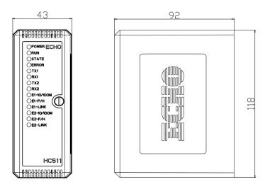
Fig. D- 1 HC511 Controller Module Panel and Dimension
