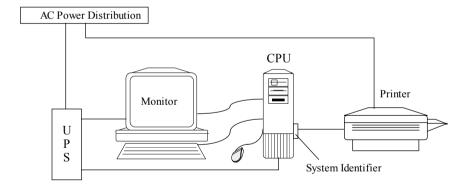
Fig. 2-18 Workstation Installation
