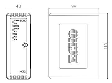
Fig. C- 5 HC121 Module Panel and Dimension
