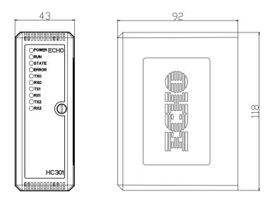
Fig. F- 1 HC301 Module Panel and Dimension
