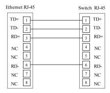
Fig. G- 7 Ethernet to Switch
