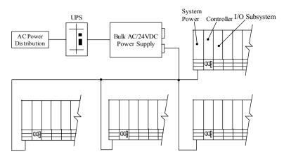
Fig. E- 3 UPS Installation for Conroller Power Backup
