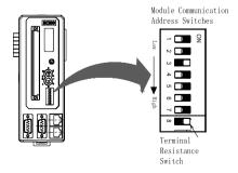
Fig. B- 8 DIP Switches Settings of module communication address
