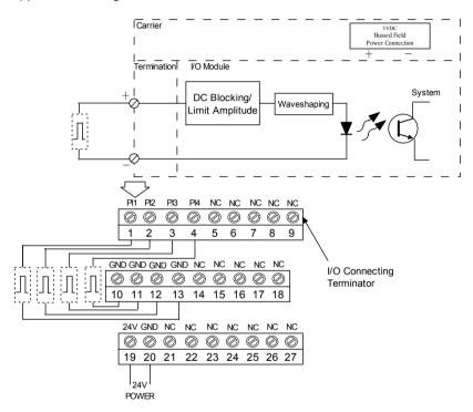
Fig. C- 12 HC141 Module Wiring Diagram
