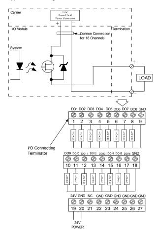
Fig. C- 10 HC133 Module Wiring Diagram
