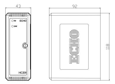
Fig. E- 1 System Power Module Panel and Dimension
