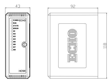
Fig. C- 1 HC101 Module Panel and Dimension
