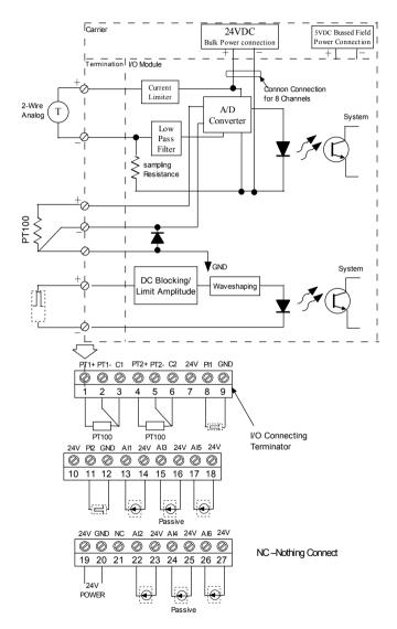
Fig. G- 8 10 Module Wiring Field
