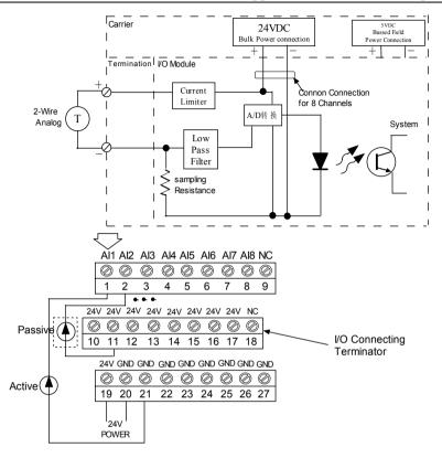
Fig. C- 2 HC101 Wiring Diagram
