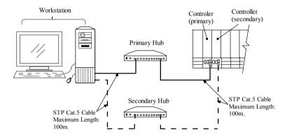
Fig. M- 1 Redundant Controller Network Example
