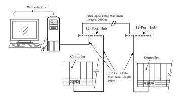
Fig. 2-21 Fiber-Optic Control Network Example
