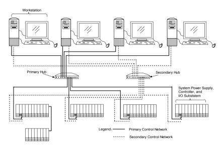
Fig. 1-5 Control Network Example (8 nodes)
