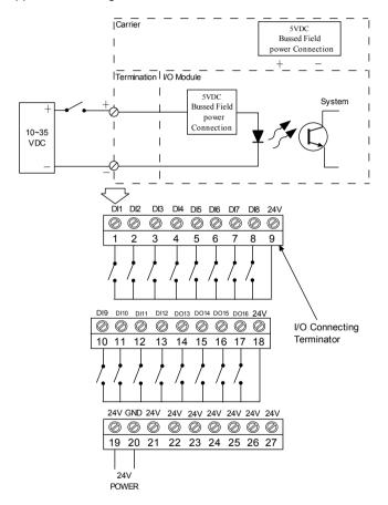
Fig. C- 8 HC112 Module Wiring Diagram
