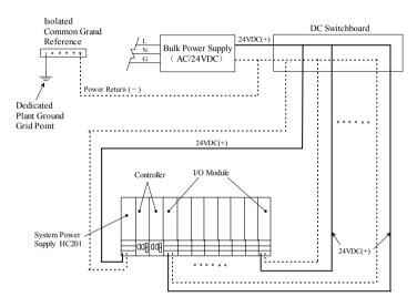
Fig. K- 1 Power Supply and Grounding
