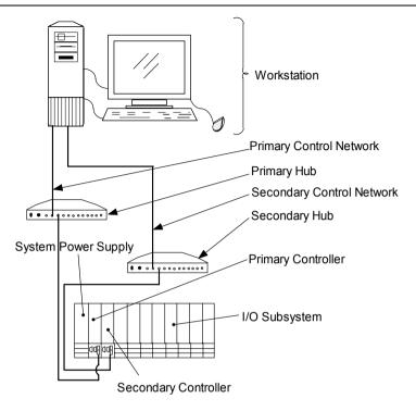
Fig. 1-1 Super E50 System Overview Diagram
