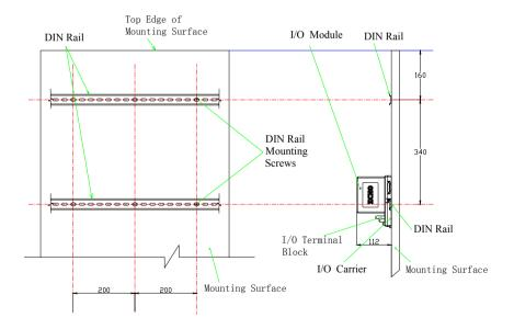
Fig. 2-7 DIN rails installation horizontally
