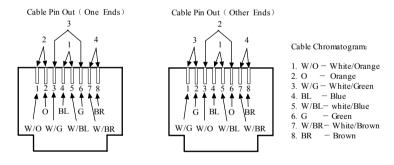
Fig. H- 2 Cable Pin Out for No Hub System
