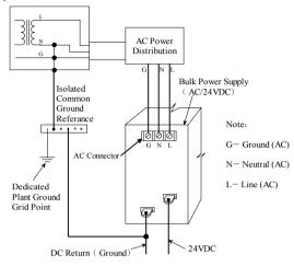
Fig. 2-23 Simplex Power and Ground Wiring Diagram fo Bulk Power Supply (AC/24VDC)
