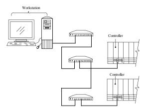
Fig. 2-20 Cascaded Hub Installation
