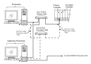
Fig. 2-22 Plant LAN Network Connections
