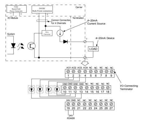
Fig. C- 6 HC121 Module Wiring Diagram
