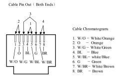
Fig. H- 1 Control Network Cable Pin Out (Both Ends)
