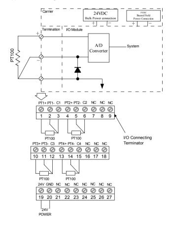
Fig. C- 4 HC104 Module Wiring Diagram
