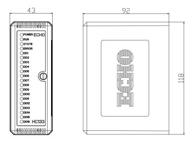
Fig. C- 9 HC133 Module Panel and Dimension
