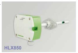
The  $CO_2$  concentration up to 10,000ppm and the temperature are available on the voltage or current analogue outputs. The HLX850 offers an additional option for a passive temperature sensor output with 2-wires connection. An optional kit facilitates easy configuration and adjustment of HLX850.
