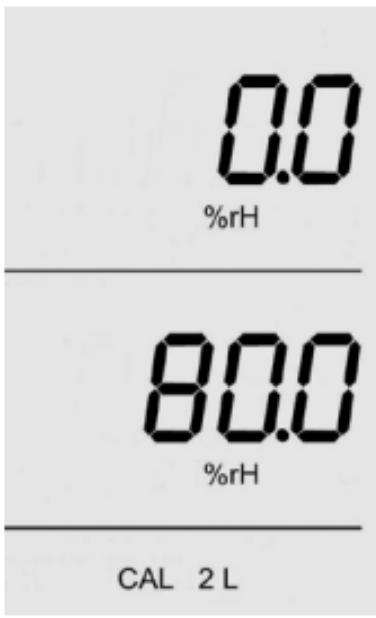
**CAL2:** With CAL2 (single-point calibration) you set the offset for Sensor 2 (rel. humidity). The offset turns the characteristic line about the lower equalisation point (11 % r.h.). The equalisation point must be in the range of 30 % ... 95 % r.h. The offset is shown in the upper half of the display. Maximum offset is  $\pm 10$  % rH. CAL2 can only be selected in connection with the unit % r.h.
