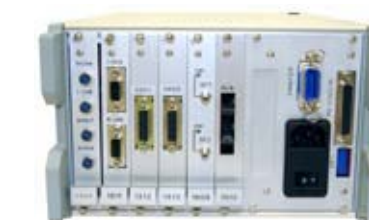
Model 1560 has 6 slots for modules
